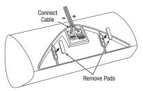
Use the supplied screws to attach the speaker to the wall-mount bracket. The screws thread into the center foot-rest openings that were exposed when you removed the rubber pads in the previous step.
