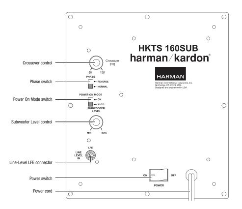
**Crossover control:** This knob adjusts the subwoofer's cutoff between 50Hz and 150Hz. The higher you set the Crossover control, the higher in frequency the subwoofer will operate and the more its bass will "overlap" that of the system's other speakers. This adjustment helps achieve a smooth transition of bass frequencies between the subwoofer and the system's other speakers for a variety of different rooms and subwoofer locations.
