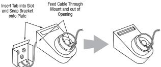
6. Fit the terminal cover onto the bracket as shown in the illustration below, then connect the speaker leads to the terminals on the underside of the speaker. Remember to observe the correct polarity.
